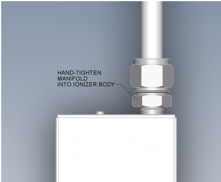
Figure 3. Outlet Manifold
